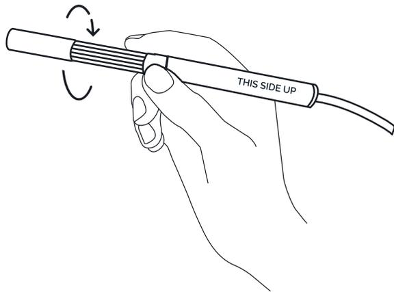
Point the hearScope at an object about 25mm from the front of the scope and adjust the focus wheel until the object is in focus to set initial focus.
