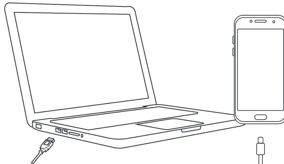
Connect your hearScope to your smartphone (use the micro USB or USB-C adapter), or to your laptop/PC (plug in the USB cable in the USB port of the laptop/PC) and grant your smartphone, laptop or PC permission to access the hearScope.
