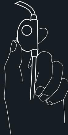
The light intensity can be adjusted by turning the wheel attached to the cable, it is recommended to turn the intensity up to maximum for first use. Use the button on the cable to assist with the capturing of images during examinations.
